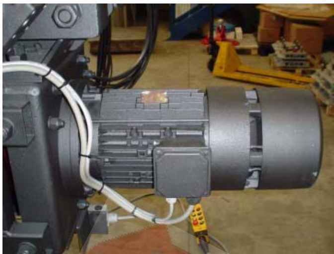
Lifting motor ELBE, self-braking type with A/C brake
